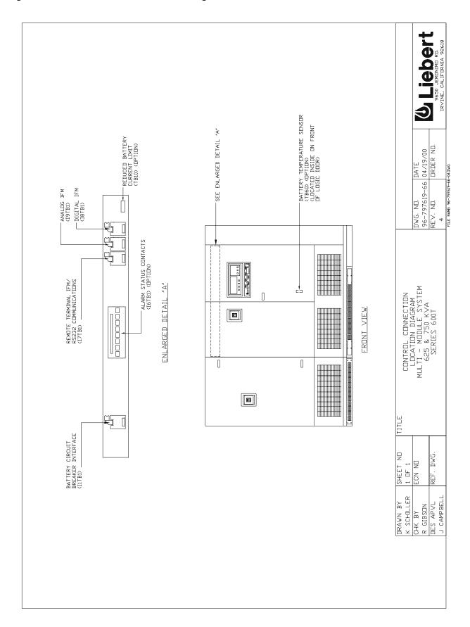
Figure 36 Control Connection Location Diagram, SCCC & SCCI
